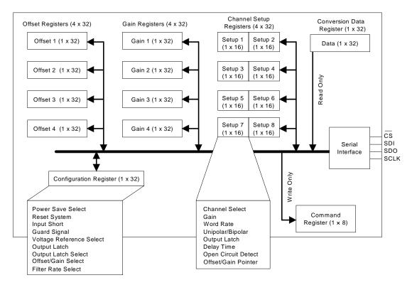
Figure 6. CS5532/34 Register Diagram
