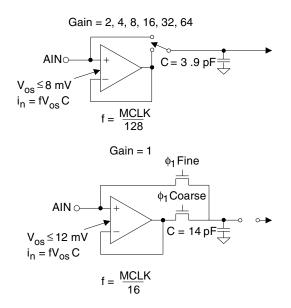
Figure 4. Input models for AIN+ and AIN- pins
