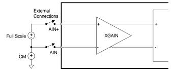
Figure 14. System Calibration of Gain
