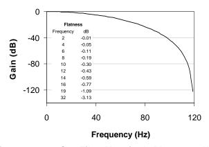
Figure 17. 120 Sps Filter Magnitude Plot to 120 Hz
