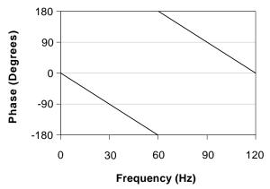
Figure 18. 120 Sps Filter Phase Plot to 120 Hz
