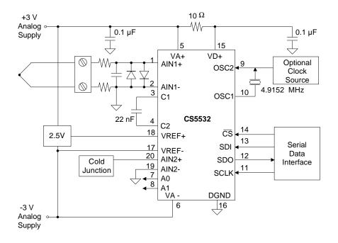
Figure 24. CS5532 Configured for Thermocouple Measurement
