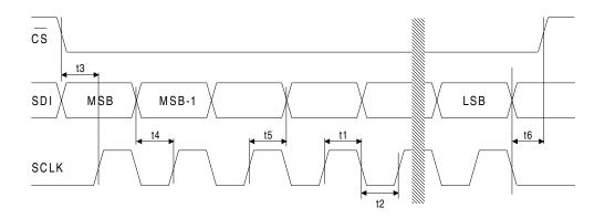
Figure 1. SDI Write Timing (Not to Scale)
