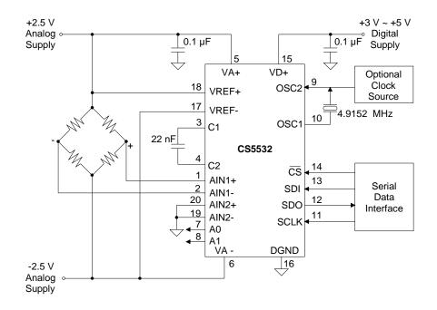
Figure 22. CS5532 Configured with ±2.5 V Analog Supplies
