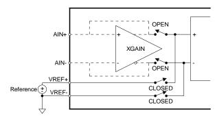
Figure 12. Self Calibration of Gain
