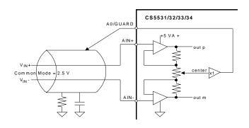
Figure 8. Guard Signal Shielding Scheme
