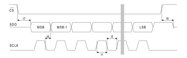
Figure 2. SDO Read Timing (Not to Scale)
