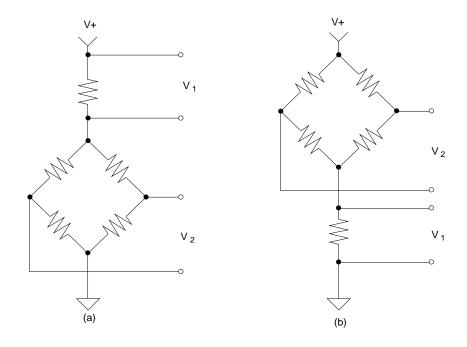
Figure 25. Bridge with Series Resistors
