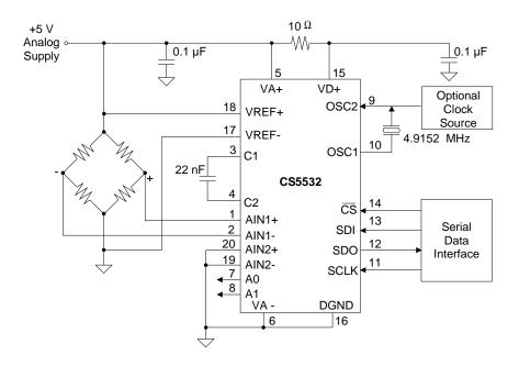
Figure 21. CS5532 Configured with a Single +5 V Supply
