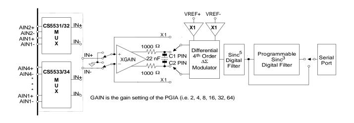
Figure 3. Multiplexer Configuration
