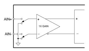
Figure 11. Self Calibration of Offset
