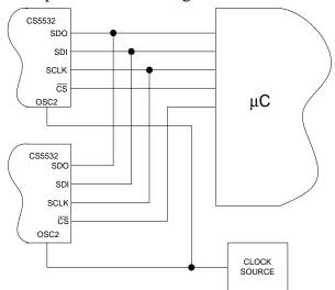
Figure 15. Synchronizing Multiple ADCs
