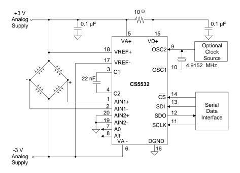
Figure 23. CS5532 Configured with ±3 V Analog Supplies
