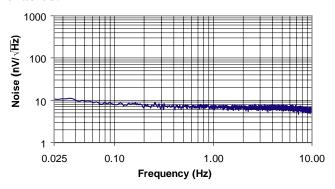
Figure 5. Measured Voltage Noise Density, 64x
